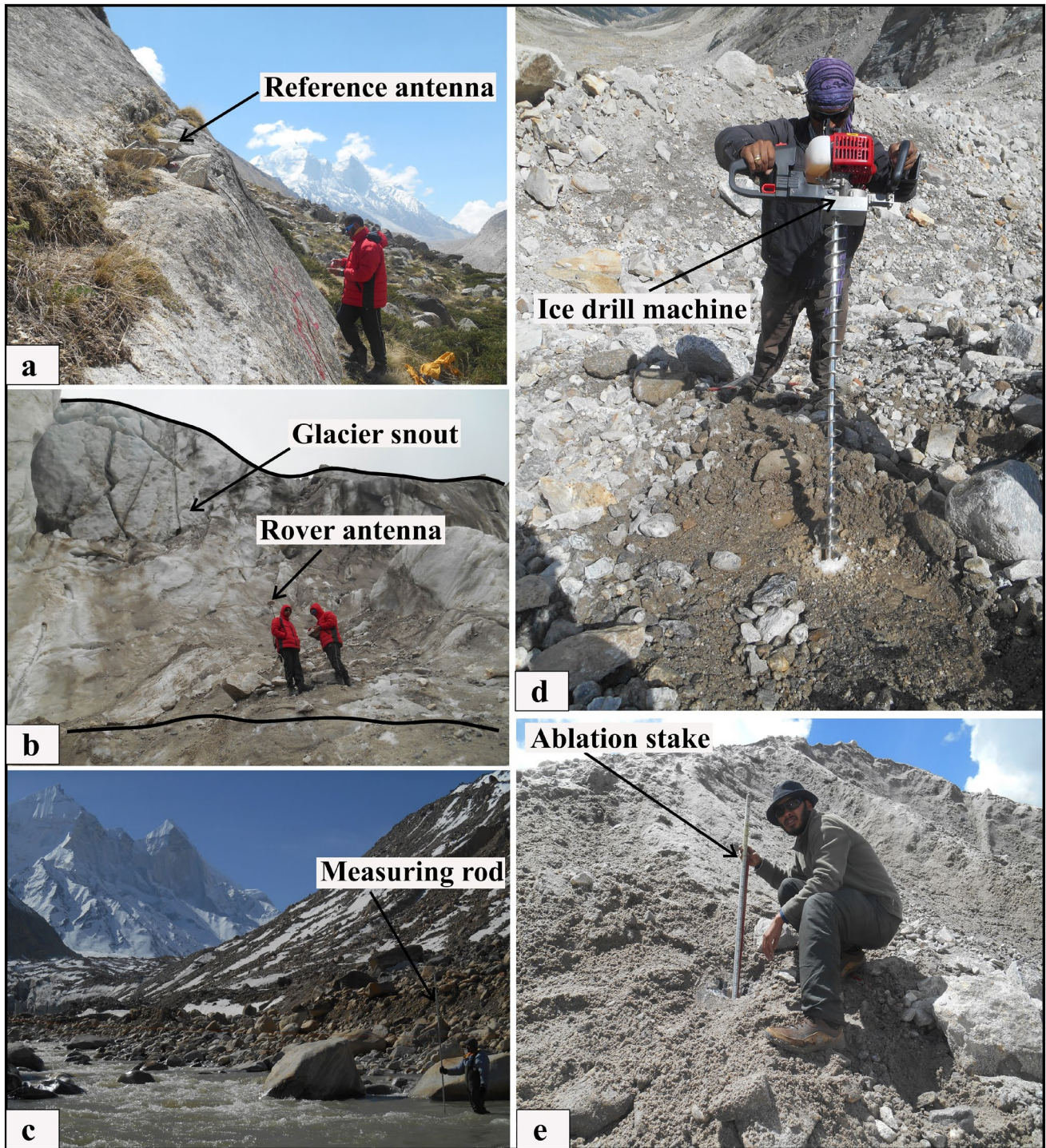
Fig. 2 a Reference antenna mounted on solid bedrock, b GPS survey along the snout of Gangotri glacier, c measurements of cross section area across the Bhagirathi stream draining from Gangotri glacier, d
