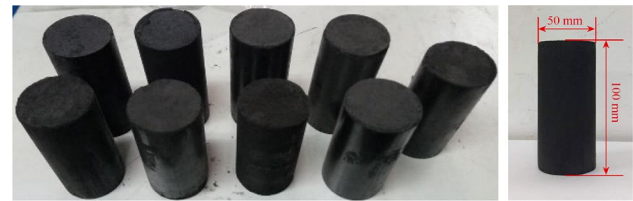
Fig. 1 Cylindrical coal samples with varying moisture content
