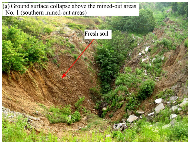
Fig. 7 Ground surface collapses above the mined-out areas
