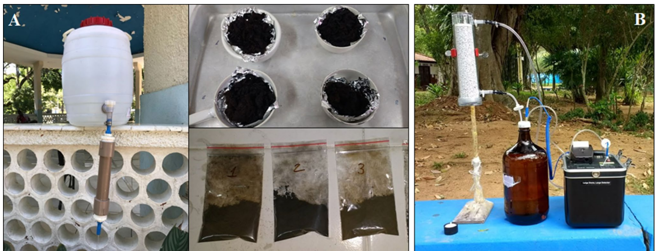
Fig. 3 a Sample preparation methodology for the ^{226}\text{Ra} and ^{228}\text{Ra} analyzes, b Big bottle system used for dissolved ^{222}\text{Rn} monitoring
