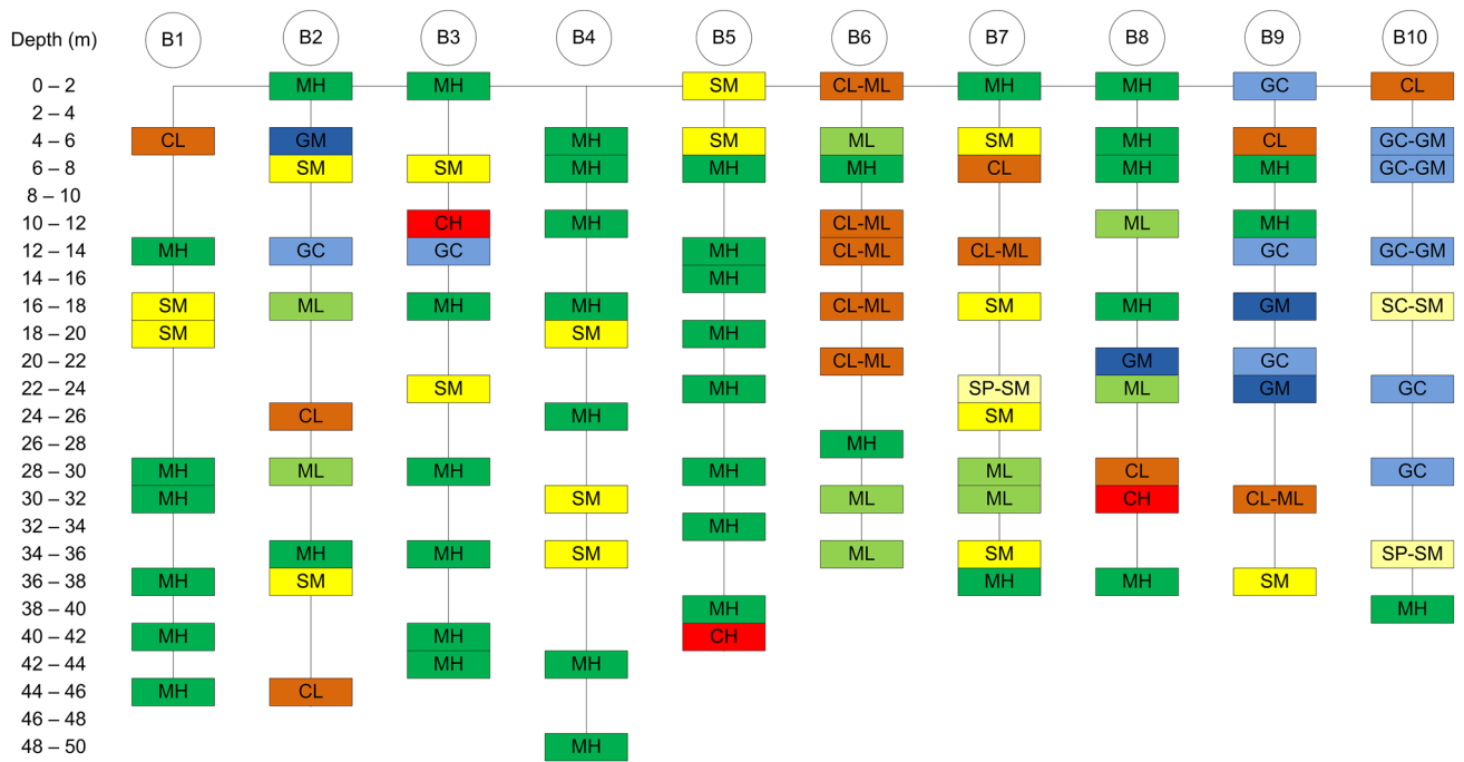
Fig. 5 USCS representation of spoil material in a lignite spoil heap in northern Greece (Zevgolis et al. 2018b)
