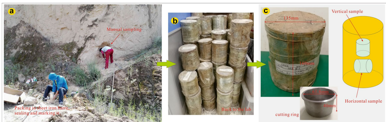
Fig. 3 Soil sampling schematic: a manual sampling, marking, and sealing of the samples; b sample transportation back to the lab; and c preparation of vertical and horizontal cutting ring samples
