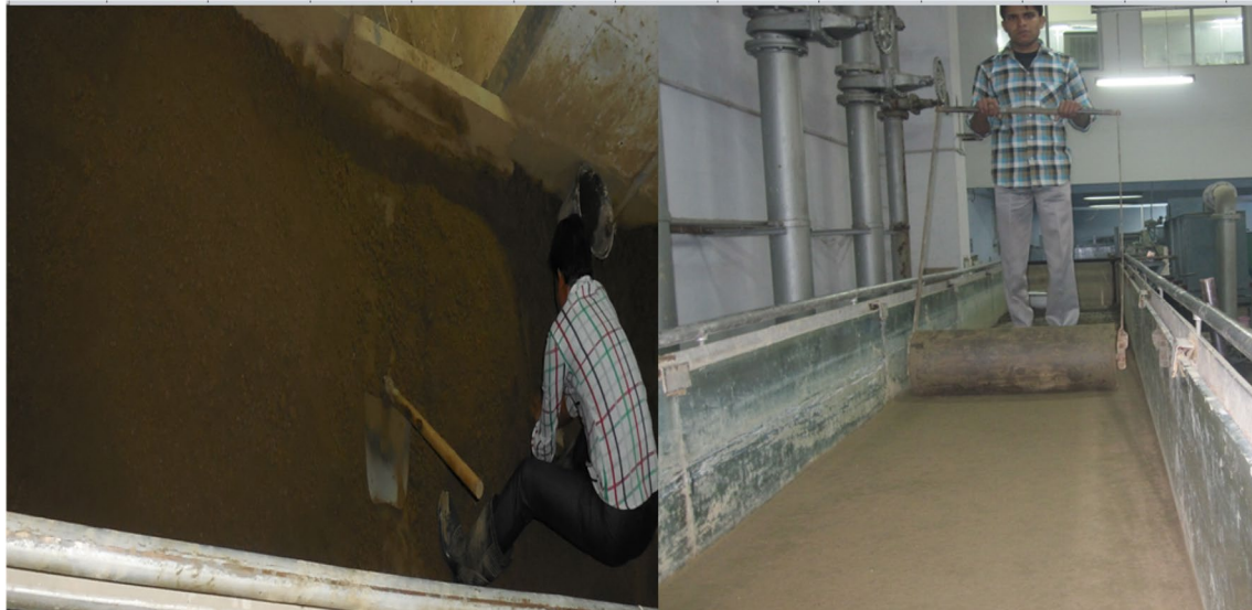
Fig. 2 Preparation of sediment mixture and channel bed
