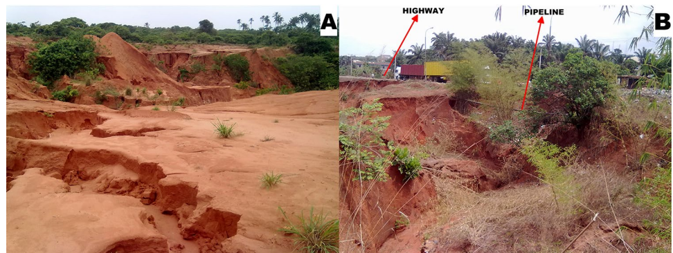
Fig. 2 Photographs of severely eroding soils due to poor urban drainage design within the study area
