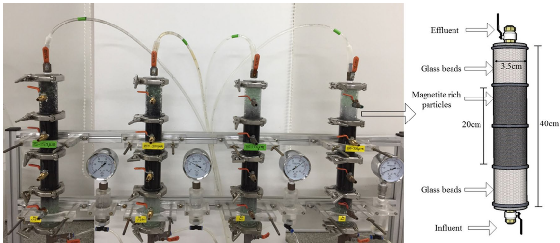
Fig. 2 Photo of the column operation with column design parameters at right side
