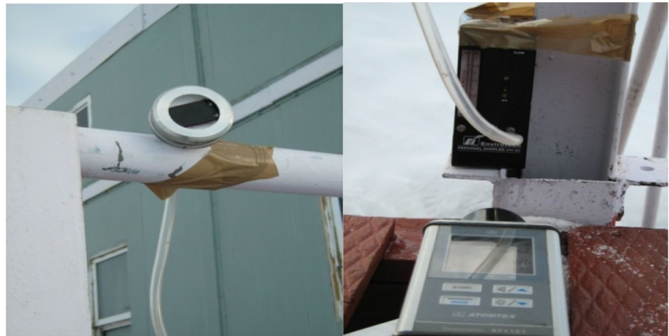
Fig. 4 Experimental set-up for the measurement of ^{222}\text{Rn}/^{220}\text{Rn} progeny concentrations in outdoor location of Maitri station using flow mode integrated sampler
