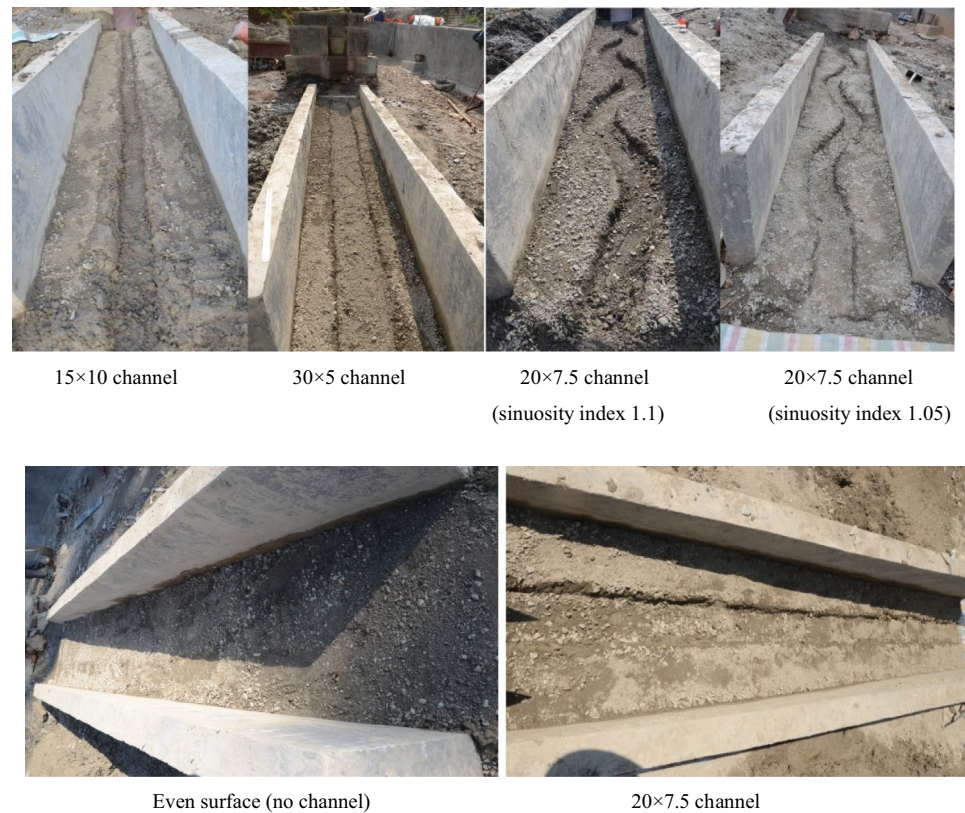
Fig. 5 Six channel morphologies set up for this experiment
