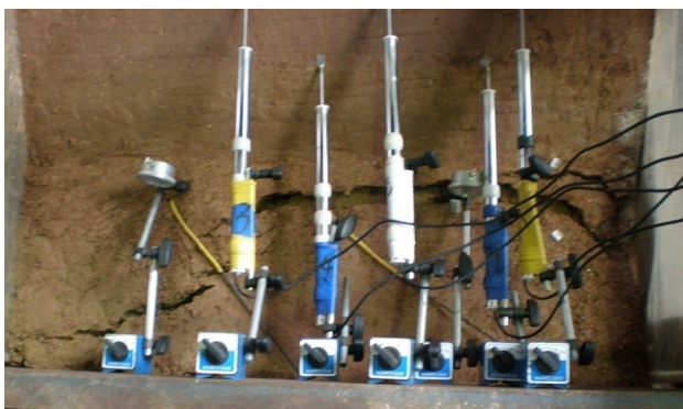
Fig. 15 Cracks of embankment in Model ④
