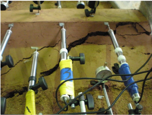
Fig. 9 Cracks of embankment in Model ①
