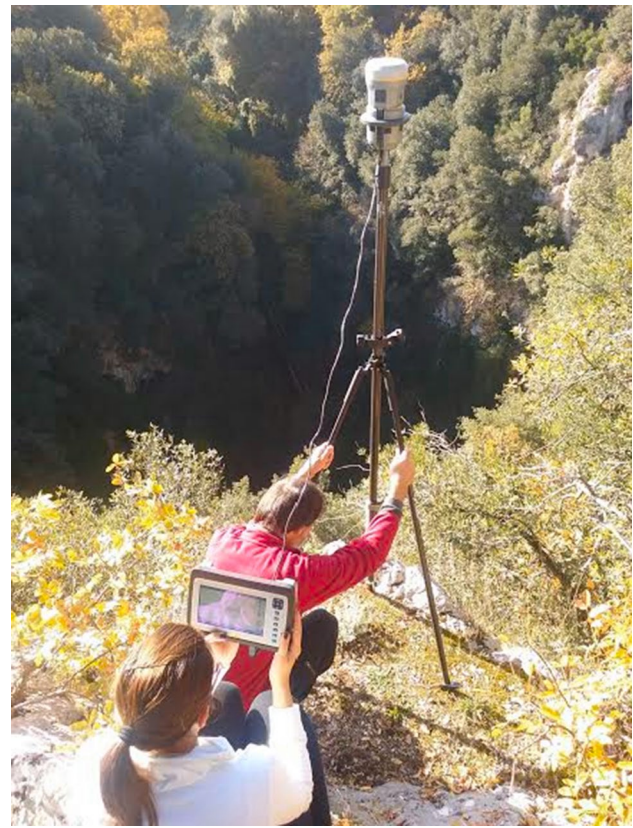
Fig. 9 The imaging rover combined with GPS/GNSS receiver (on top)
