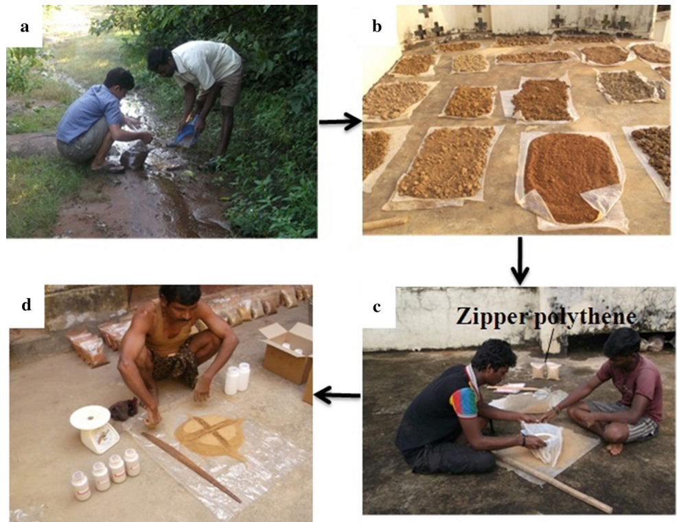
Fig. 4 Photographs showing procedure from collection of geochemical sample to preparation of sample for chemical analysis. a Collection of stream sediment sample (unit cell sample) from a stream in the study area. b Sun drying of collected unit cell samples by putting in transparent polythene sheet at the field camp. c Sieving of dried unit cell samples through – 120 mesh sieve and subsequent storage of sample in zipper polythene in the field camp. d Preparation of composite cell samples by through mixing of unit cell samples followed by coning and quartering and weighing. Finally, samples are stored in labelled bottles for chemical analyses and future reference
