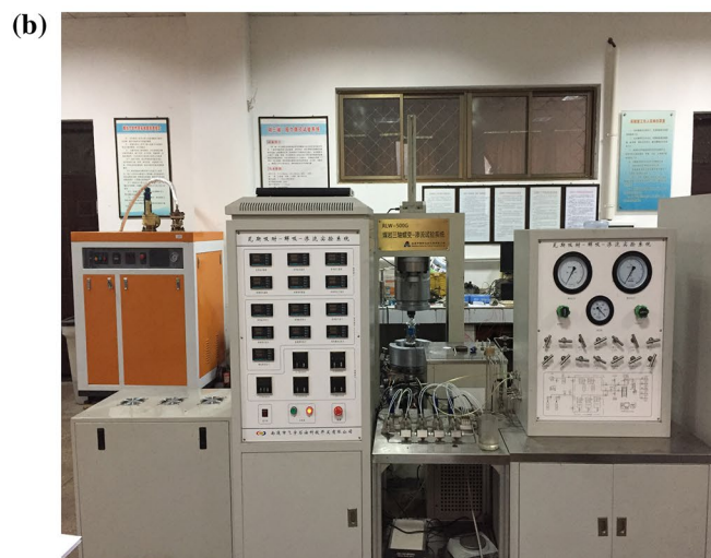
Fig. 4 Triaxial creep–seepage experimental system a Schematic diagram of testing system. b The map of testing system
