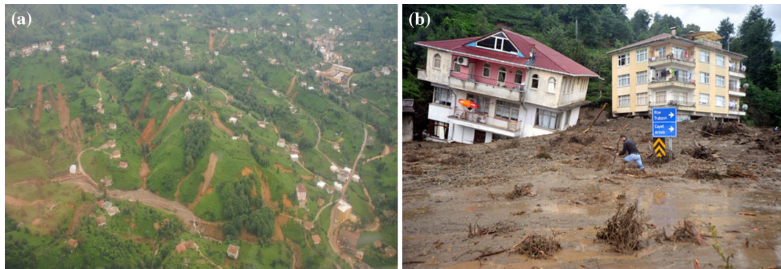
Fig. 1 a Aerial view of numerous shallow landslides after an intense rainfall in the city of Rize, Turkey, b damage due to landslide after heavy rainfall in Rize, northern Turkey, in August 2010
