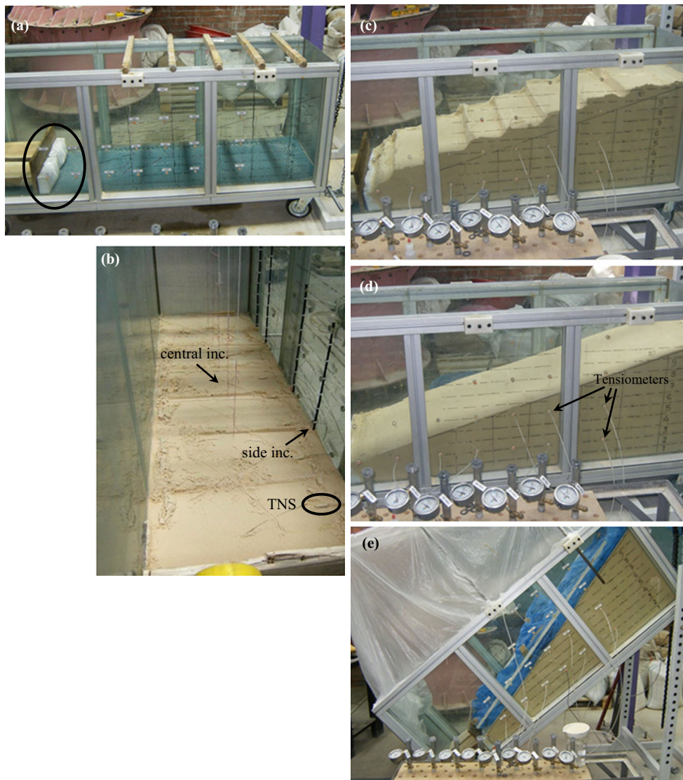
Fig. 6 a Filter material located at the toe of the slope and geonet at the bottom boundary of the flume, b central and side inclinometers (hanging from wooden bars above the flume throughout soil placement) and miniature tensiometer placement (tensiometers are placed at two different locations: one group near the glass face of
