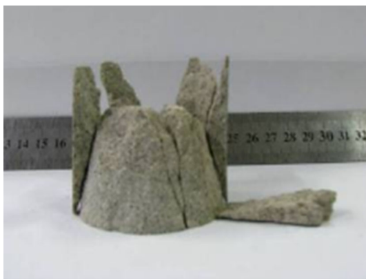
Fig. 5 Typical failure pattern of sandstone under dynamic loading after confining pressure unloading (Yin et al. 2012b)
