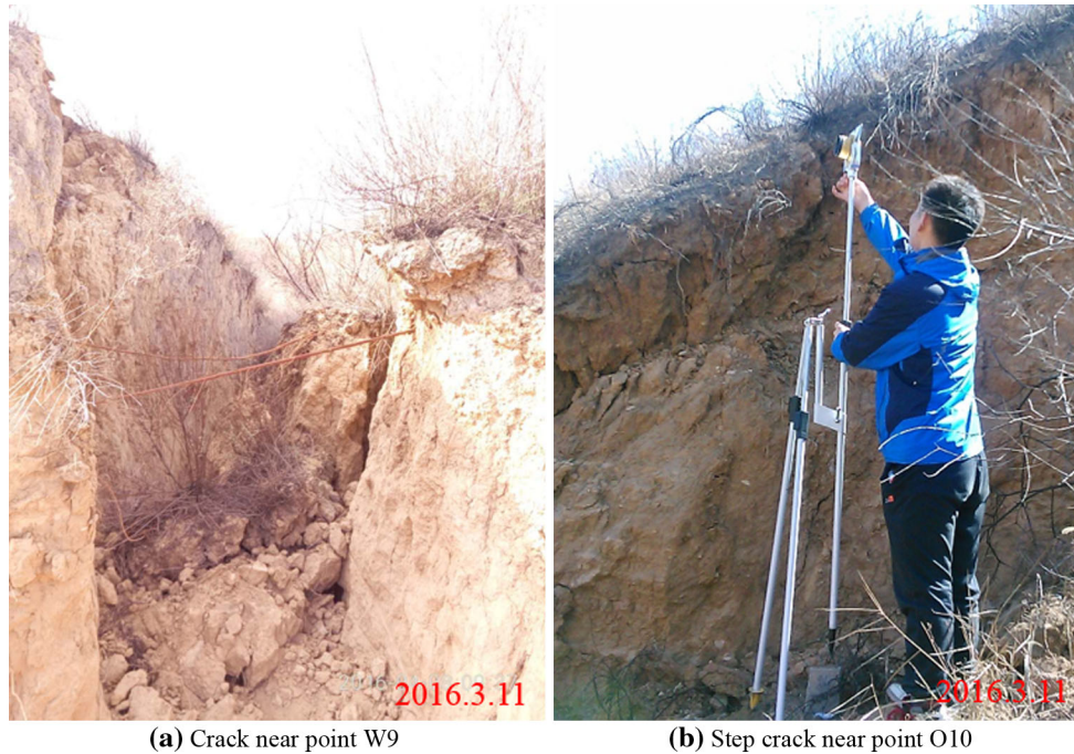
Fig. 9 Surface step cracks caused by underground mining
