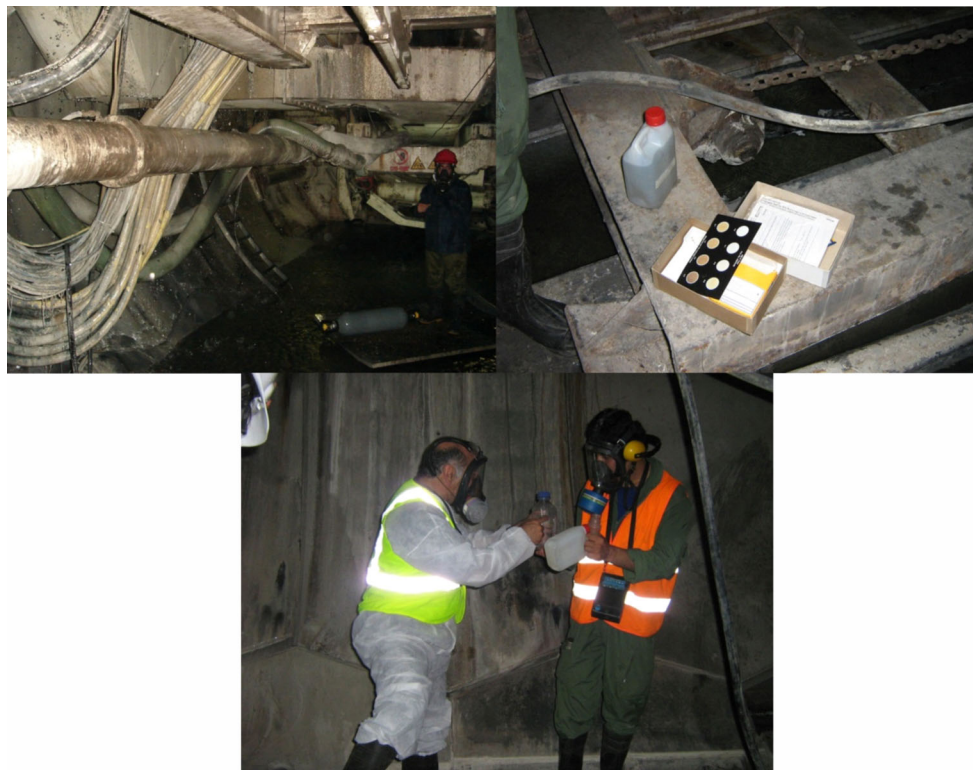
Fig. 3 Gas sampling with vacuum capsule and sampling of gas dissolved in groundwater inflow in the Aspar tunnel
