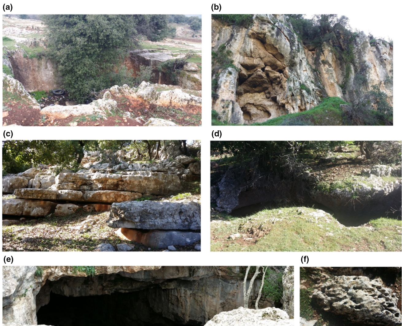
Fig. 4 Karst features within the catchment area (based on the geological survey for the area); a doline ( \sim 15 \times 10 m), b dissolution in the rocks, c big fractures between beddings planes, d , e caves, and f dissolution and big pores inside the rocks
