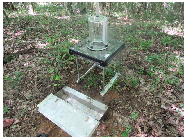
Fig. 3 Field experiment setup with portable rainfall simulator and Gerlach trough
