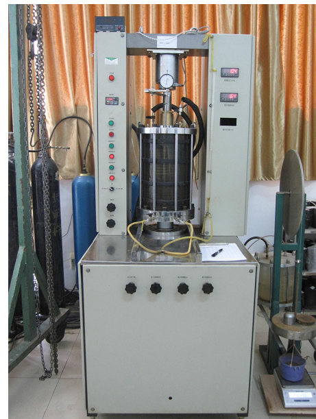
Fig. 5 YLSZ150-3 stress-controlled machine
