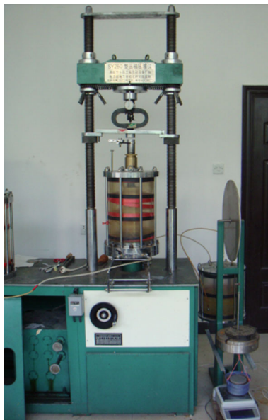
Fig. 4 SY250 strain-controlled machine
