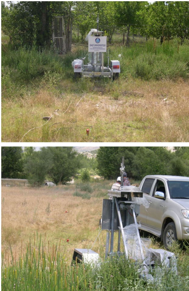
Fig. 2 Photographs of the trailer mounted drop weight source utilized during the MASW survey
