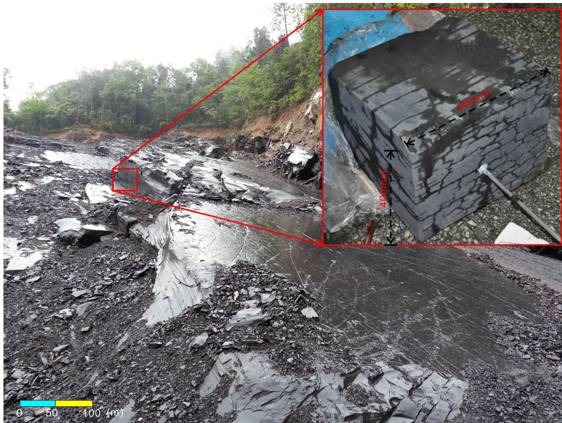
Fig. 3 Outcrop of Silurian Longmaxi shale formation in the southeastern Sichuan Basin. The water injection test is used to seek the natural fractures. Two sets of orthorhombic natural fractures were
