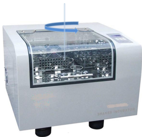
Fig. 1 The incubator shaker used for microorganism cultivation and bioleaching
