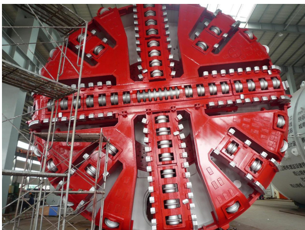
Fig. 4 Cutter head of the TBM
