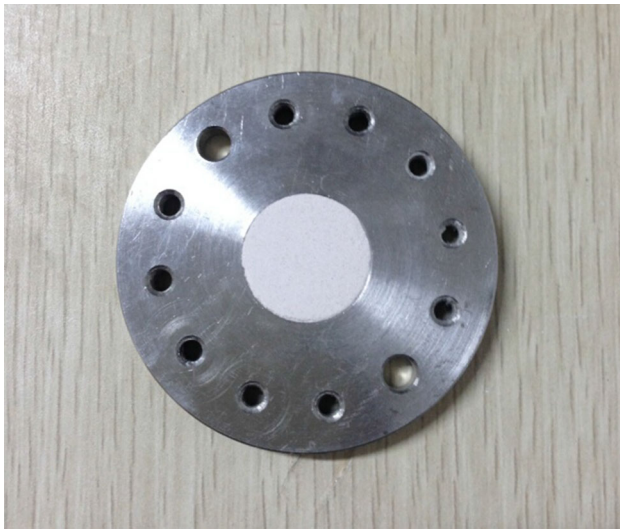
Fig. 2 The compacted GMZ bentonite with a dry density of 1.70 \text{ Mg/m}^3
