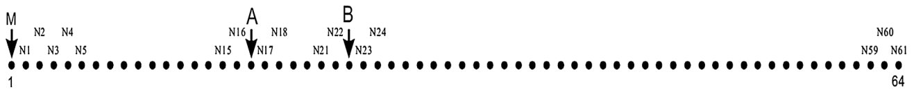
Fig. 4 61 Channel ERT data acquisition field setup using 64 electrodes, of which two as current electrodes (A, B) and one as common reference electrode (M) and 61 potentials relative to M on remaining electrodes
