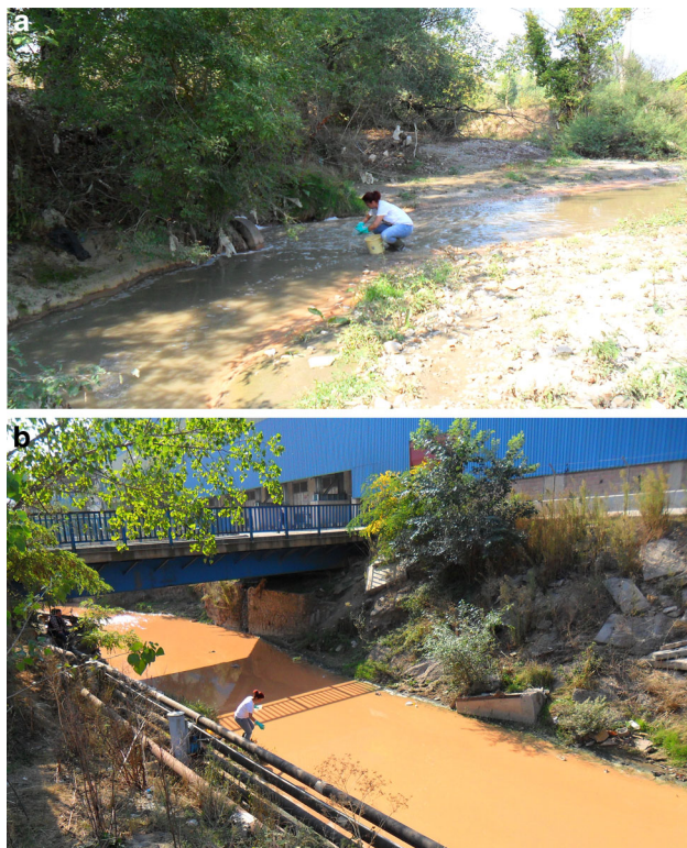
Fig. 4 A view from a D3 and b D8 surface water sampling points along Dil stream. Note turbidity and coloring in stream resulting from Değirmen stream at Dil stream intersection (D3) and near iron–steel factory (D8), respectively
