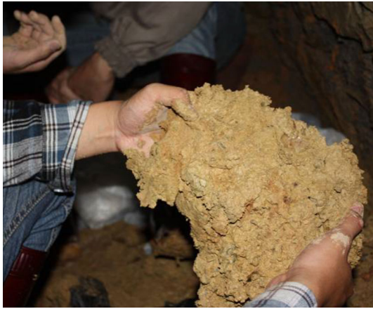
Fig. 5 Undisturbed sliding soil (samples #1 and #2)
