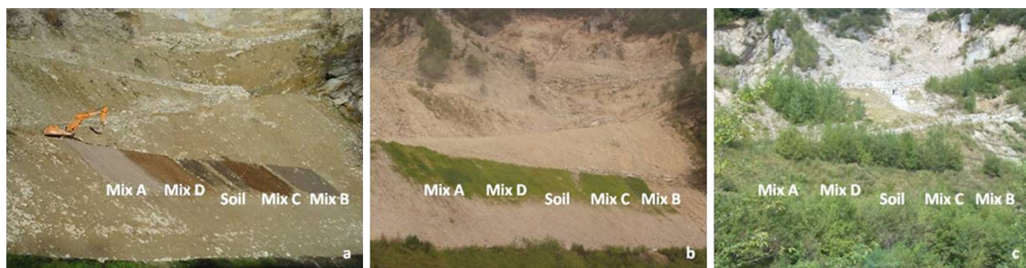
Fig. 4 Scheme of plots present on the hill side of “Cava del Tiglio” Loc. Pra del Tomo—Rorà, Turin (44°47’36”N 7°11’07”E). a 1st step of quarry rehabilitation; b plant growth 3 months after seeding; c quarry rehabilitation after 8 years
