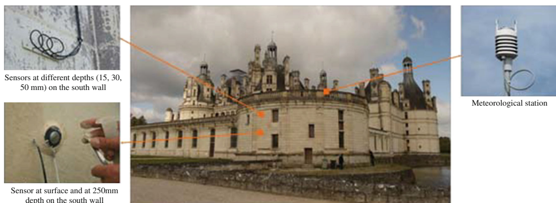
Fig. 3 The meteorological station above the east tower and the sensors positioned on the south wall
