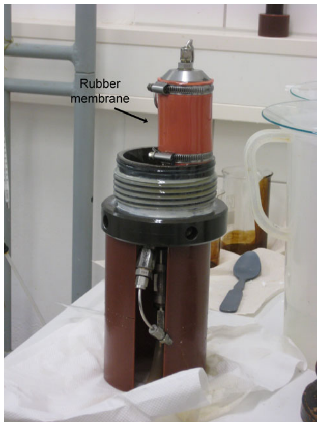
Fig. 2 Core sample wrapped in a rubber membrane and placed in a vessel filled with oil to apply the containment pressure
