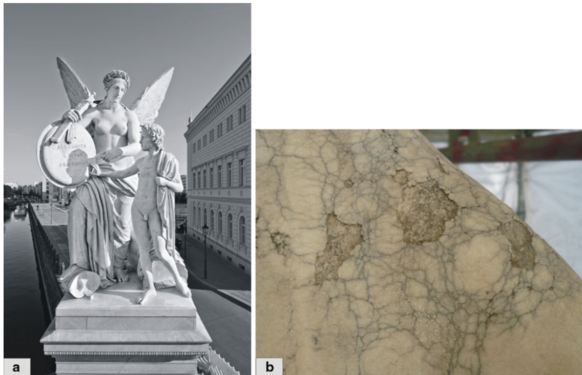
Fig. 2 a Marble Statuary from the Schlossbrücke, Unter den Linden (Berlin, Germany) “Nike instructs a boy in heroic history” by Emil Wolff 1847 and b damage phenomena of intensive cracking and network of cracks (craquelling)
