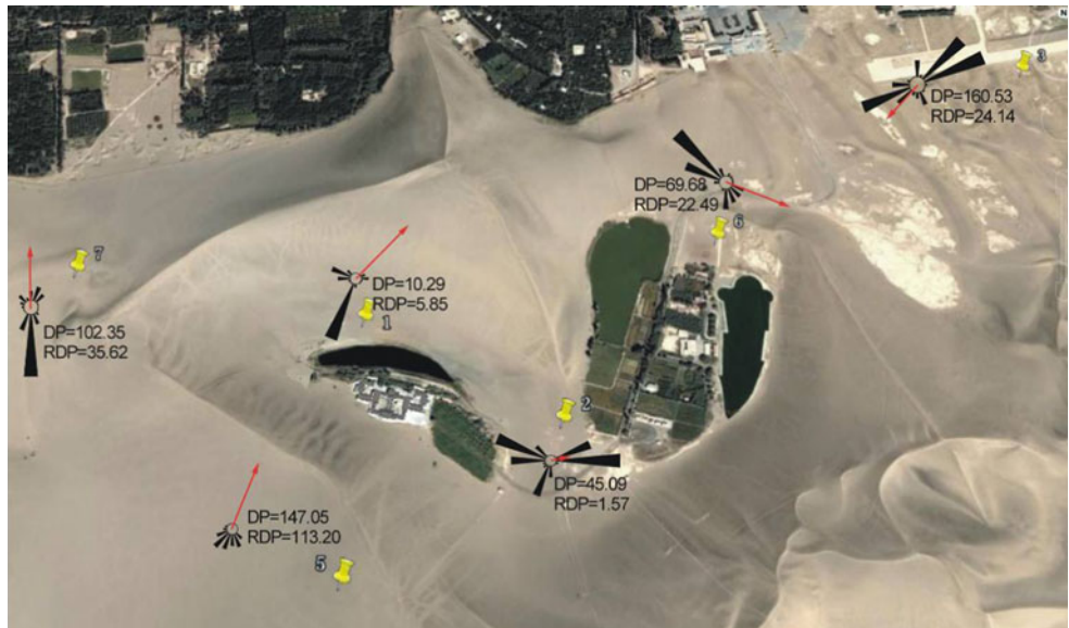
Fig. 5 Drift potential (DP) roses for the area around the Crescent Moon Spring
