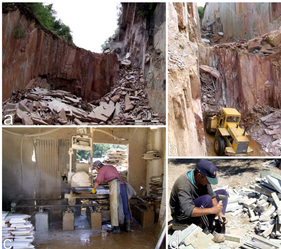
Fig. 18 Mining activities in a typical dolomitic slate quarry in the Arroyo Minas Viejas district (AMVD) in Uruguay (Company Carmine Rufo). a Active slate quarry where Piedra laja ocre (U38A) is mined. b Active slate quarry where Piedra laja gris plomo
