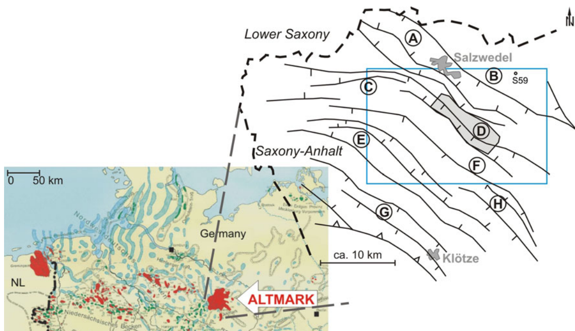
Fig. 1 Map of central Europe, covering the northern part of Germany and the western part of the Netherlands and showing major gas fields (in red) and Zechstein salt structures (in dark blue) (after LBEG 2010). Also shown is the area of the Altmark gas field with its different compartments (sub-fields): A Salzwedel, B Riebau,
