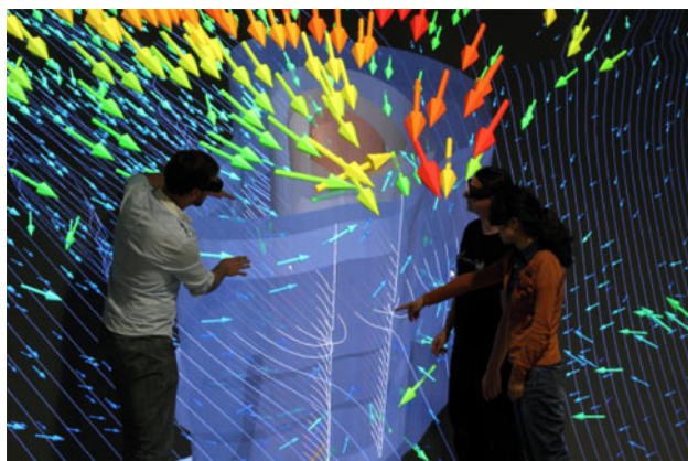
Fig. 13 Streamlines captured by the triple pumping wells and the groundwater flow velocity shown in a virtual 3-D environment
