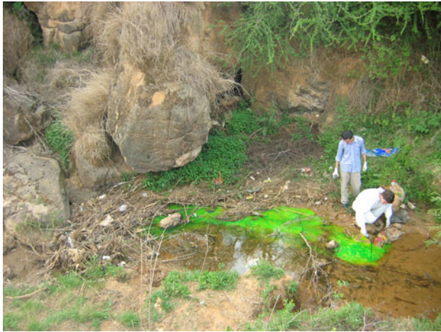
Fig. 8 Injection of uranine in Qiaotou Ponor
