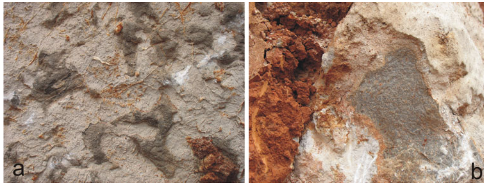
Fig. 5 In some places, lenses of dolomitized limestone ( dark gray ) measure up to several dm 3 in volume (width of view is 25 cm) ( a ). Weathered rock is more than 5 cm thick in places (width of view is 20 cm) ( b )
