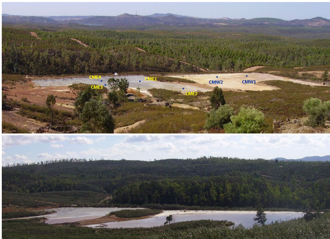
Fig. 3 Cueva de la Mora impoundment in summer ( up ) and in winter ( down ). Note the grey colour of the eastern body ( left ) and the yellow colour of the western body ( right ). Sampling points are marked on the
