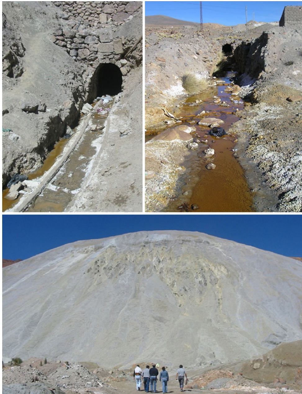
Fig. 2 AMD source 1C ( top left ), which is an active mine portal on the north slope of Cerro Rico. AMD source 1A ( top right ), which is an abandoned mine portal near the eastern base of Cerro Rico. A portion of the Pailaviri tailings deposit ( bottom ) which lies <100 m
