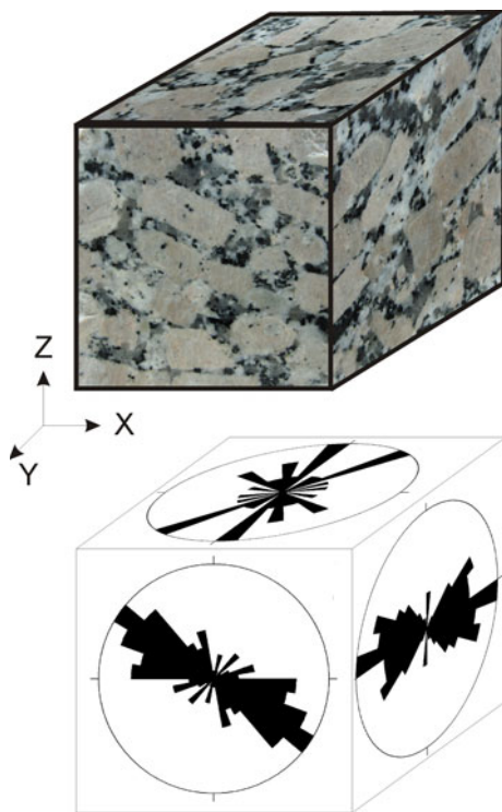
Fig. 7 K-feldspar orientation in R granite. XZ and YZ planes show the most quantity of oriented crystals with 92 and 65 measurements, respectively. In the XY slab, only 18 oriented K-feldspar were found. The slab with the greatest bowing followed the YZ plane and showed K-feldspar parallel to the Y axis
