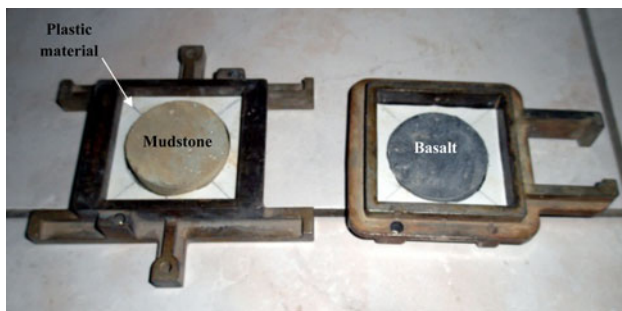
Fig. 9 Shear box test samples to determine the basic friction angles between basalt and mudstone
