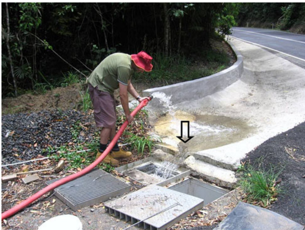
Fig. 2 Kuranda Range Road testing site at Streets Creek (during testing of sampling system). Road runoff samples were collected in a concrete gully from a 30 m long by 6.6 m wide section of road. The sample intake point was at the end of the gully (arrow). Sampling events were triggered by a water level probe installed in a V-notch weir downstream of the intake point (not shown)
