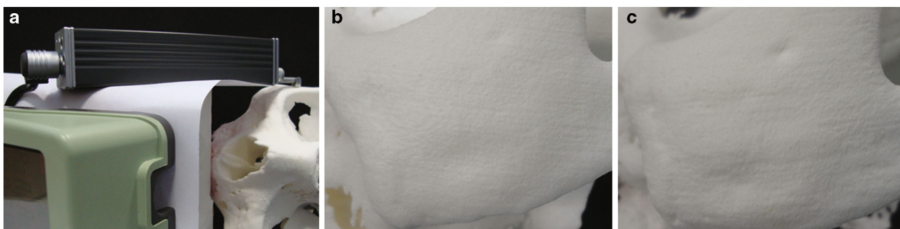
Fig. 2 a The roughness meter used showing how the surface roughness was measured; and two 3D models: b greatest surface smoothness CT 64 1.25, and c greatest surface roughness CB 0.25 voxel
