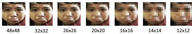
Fig. 1 Example of face images at various resolutions ranging from 48 \times 48 to 12 \times 12
