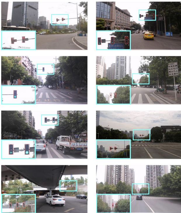
Fig. 7 Samples of traffic light detection result. The detected traffic lights are marked by red rectangles
