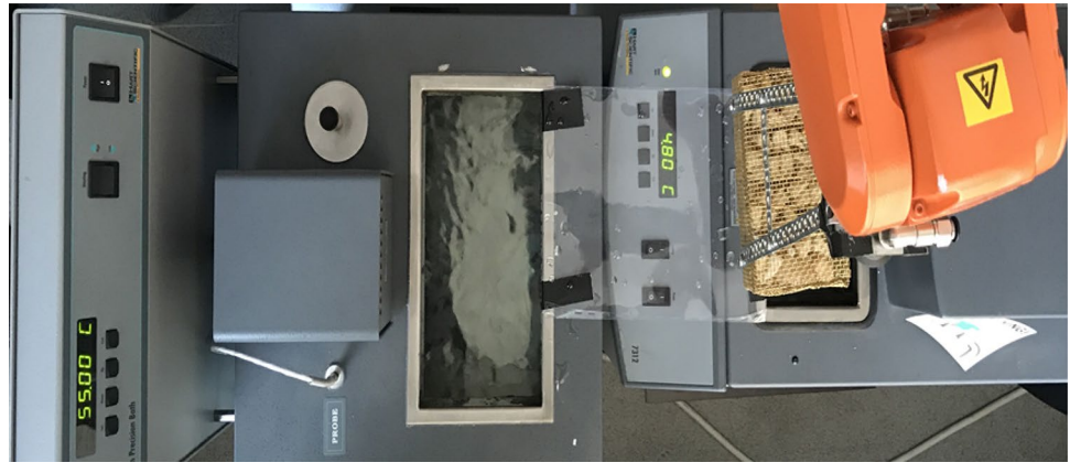
Fig. 1 Submersion rig made from ABB robot and two “Hart Scientific” thermal baths
