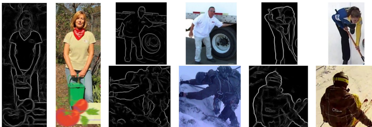
Fig. 7 Edge maps of some sample images. This type of lower-level feature can provide helpful cues for human pose estimation and discard the misleading image feature, like color, texture, etc., in the model learning process
