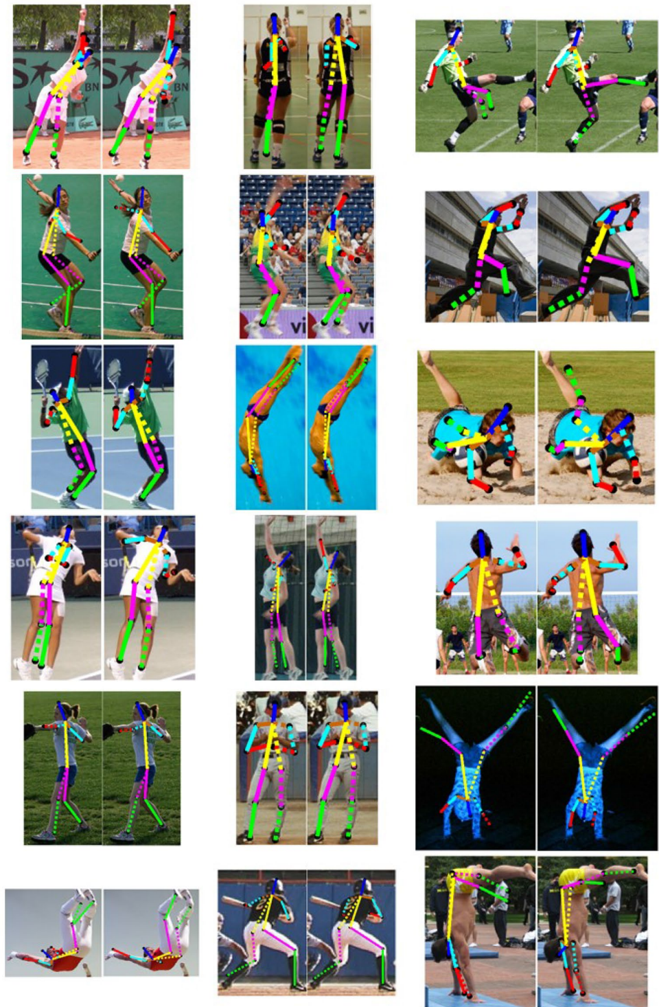
Fig. 9 Qualitative comparison between the part-based approach with and without using the edge map along with the input image. In each pair, the left and the right images show the results of the input data as RGB and RGB-E (RGB + edge map) in order. Incorporating the lower-level edge feature improves the performance of the network
