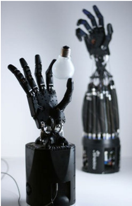
Fig. 5 Robotic hands with 5 fingers. Shadow hand [The Shadow C6M Smart Motor Hand in front of the Shadow C3 Dexterous Air Muscle Hand ( http://www.shadowrobot.com/gallery.shtml?gallery=handC6M_20091aunch&img=20090818-C6M_holdingLightBulb_frontC3blurred.jpg ) by Shadow Robot Company with license CC BY-SA 3.0 ( https://creativecommons.org/licenses/by-sa/3.0/ )]
