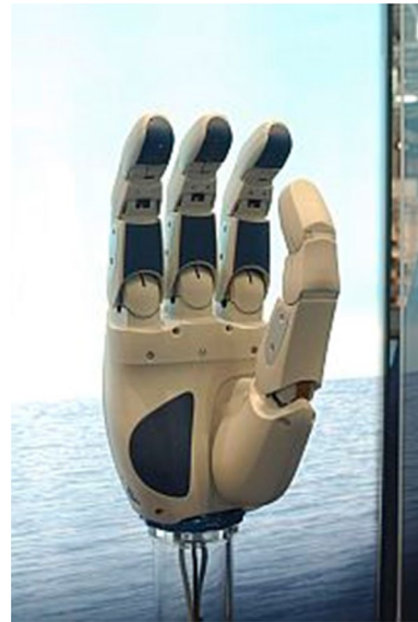
Fig. 4 Robotic hand with 4 fingers. DLR-HIT hand [DLR/HIT Hand ( https://www.dlr.de/rm/en/desktopdefault.aspx/tabid-9467/16255_read-8918/ ) by German Aerospace Center with license CC BY 3.0 DE ( https://creativecommons.org/licenses/by/3.0/de/deed.en )]
