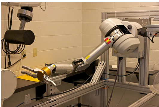
Fig. 3 Robotic hand with 3 fingers. Barrett hand [Barrett WAM arm ( https://www.flickr.com/photos/jiuguangw/6265558050/ ) by Jiuguang Wang with license CC BY-SA 2.0 ( https://creativecommons.org/licenses/by-sa/2.0/ )]
